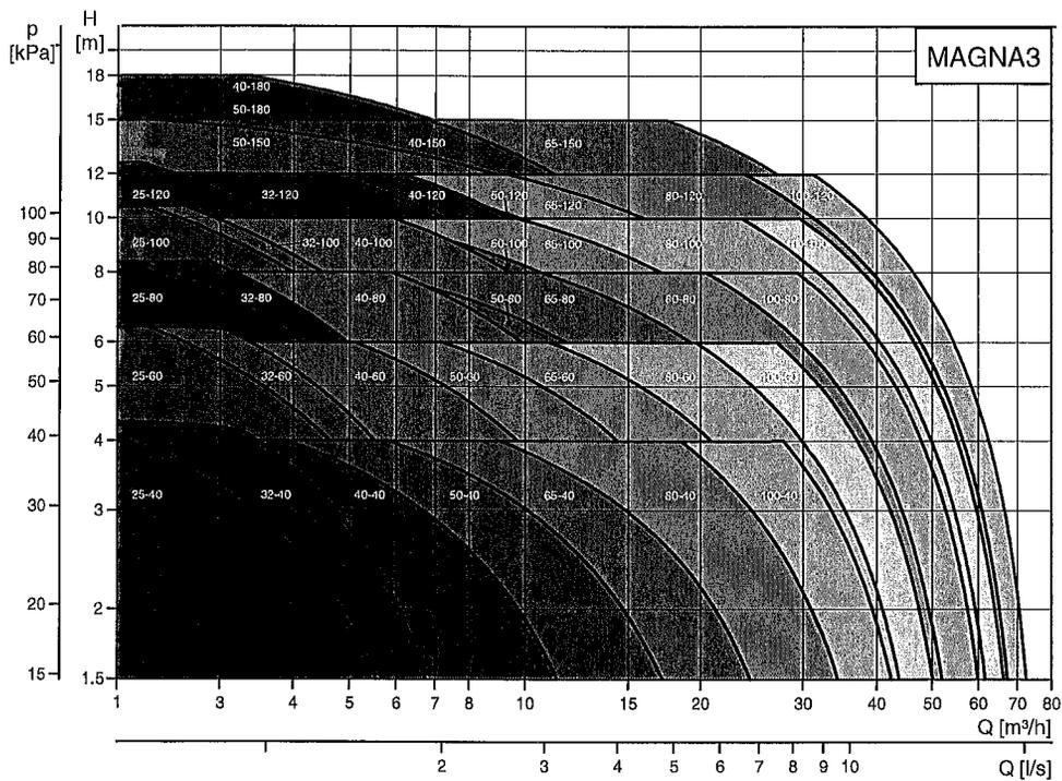
**Note:** MAGNA3 32-120 is available for flange connection and for threaded connection, but with different performance.
